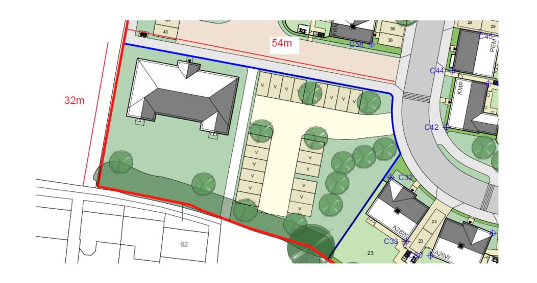
D2 Area boundary approx. 32 + 54 +10 + 15 +50 = 161m less fence between old and new areas = 129m. If high fence is removed between old and new areas and refitted to pound close side. The amount of fence would be as follows
